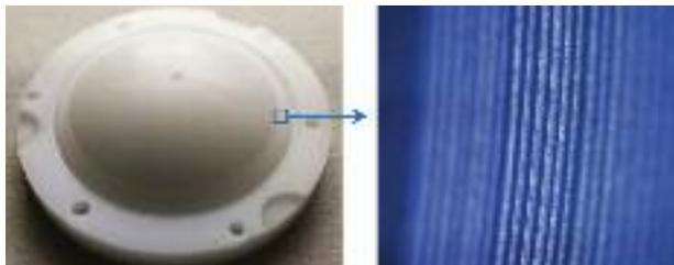
Mold (left) used to produce micro texture (right) into the edge of tag suction cups.
