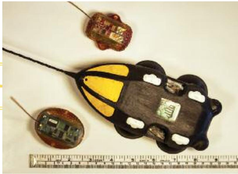
Size comparison of tags: SPOT6 location tag (top), DTAG-3 acoustic and multi-sensor (middle) and SPLASH10 location and dive data tag (bottom).
