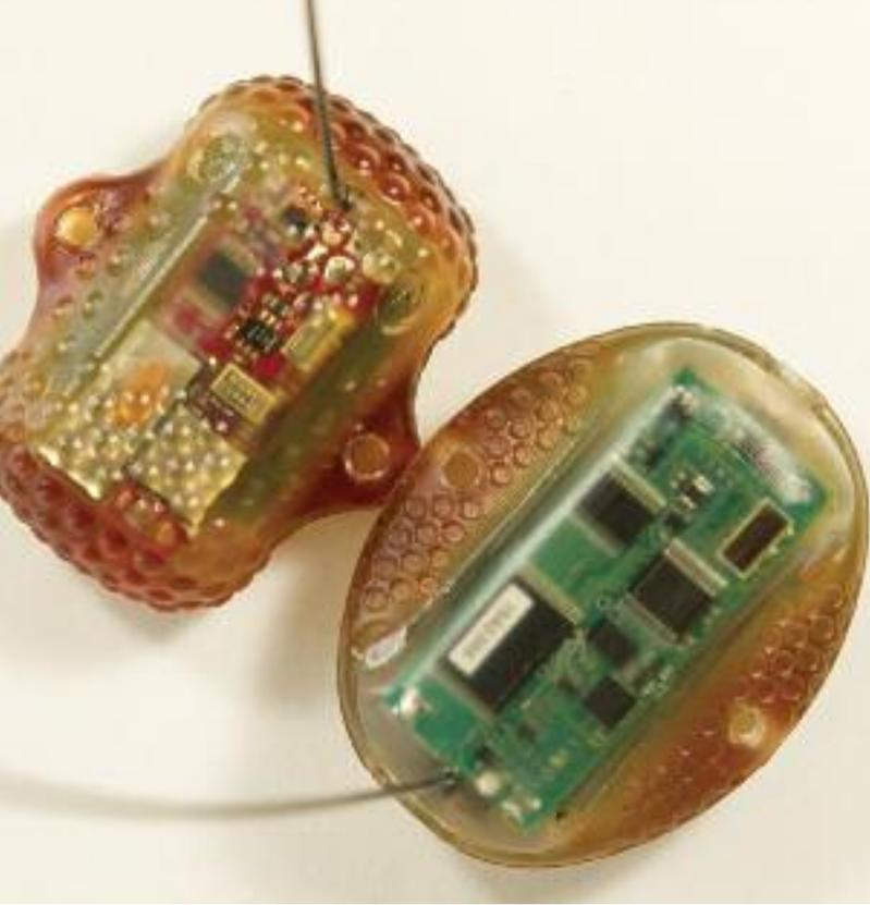
Two Low Impact Minimally Percutaneous Electronic Transmitter (LIMPET) tags that have been used in Navy-funded monitoring are the SPOT6 (left) and SPLASH10 (right) from Wildlife Computers.
