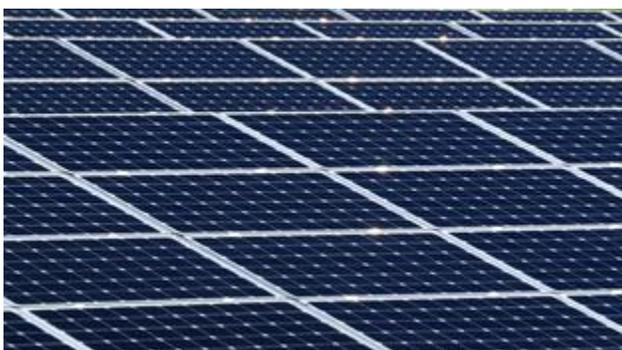
\*Solar panels produce DC energy, which is converted to AC for grid consumption.
